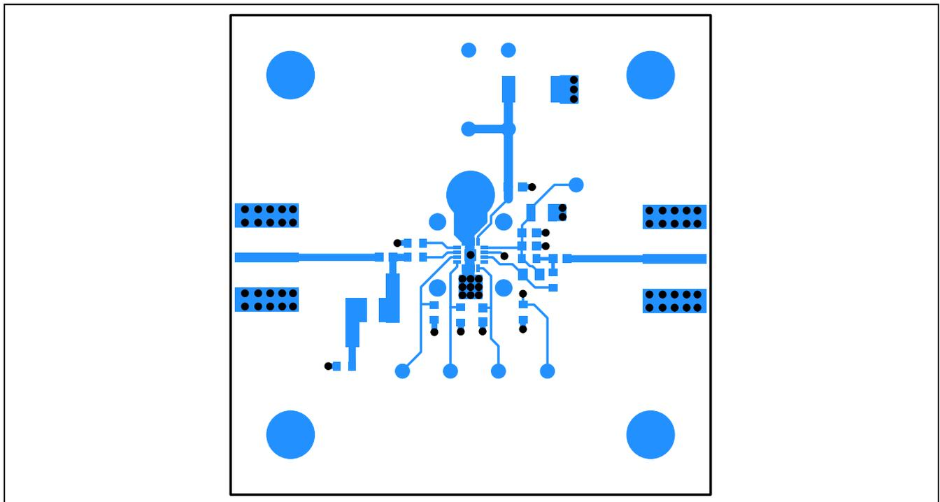
Figure 3. MAX2181 EV Kit PCB Layout—Top Copper
