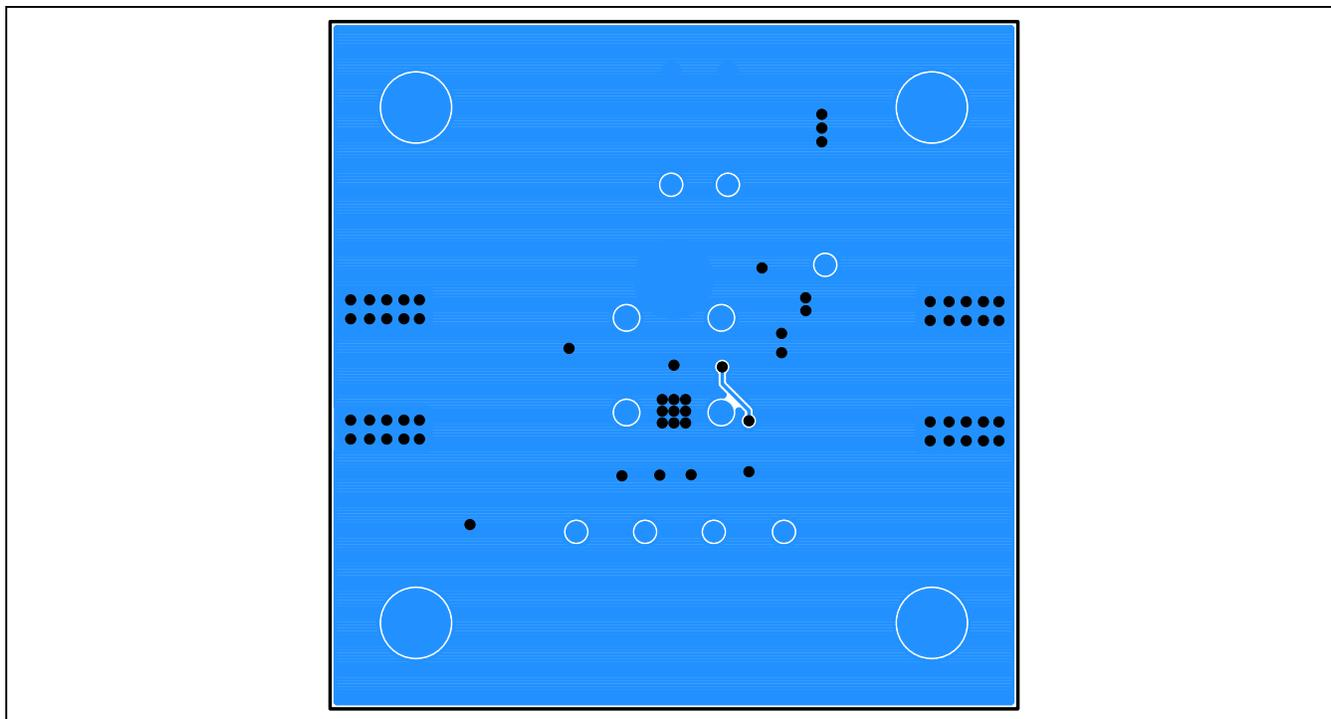
Figure 4. MAX2181 EV Kit PCB Layout—Bottom Copper
