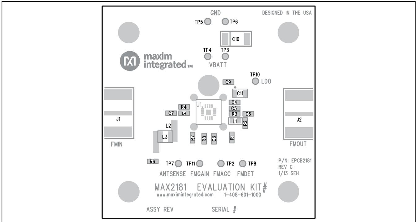
Figure 2. MAX2181 EV Kit Component Placement Guide—Top Silkscreen
