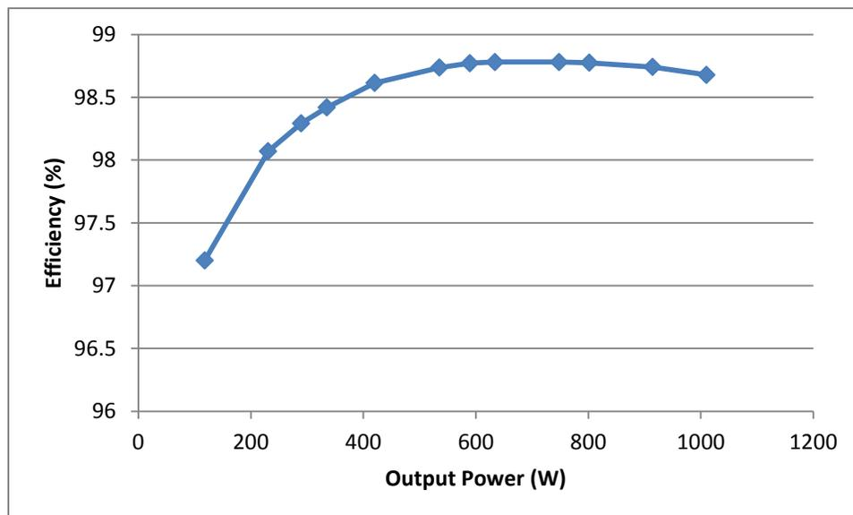
Figure 9: efficiency for a boost 200V:400V converter
