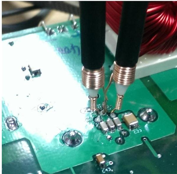
Fig. 8. Low-inductance probing of fast, high-voltage signals
