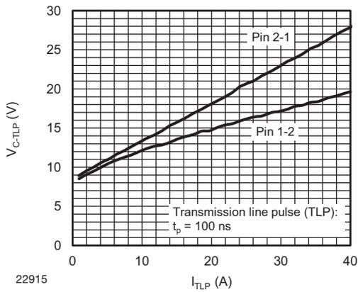
Fig. 4 - Typical Clamping Voltage vs. Peak Pulse Current
