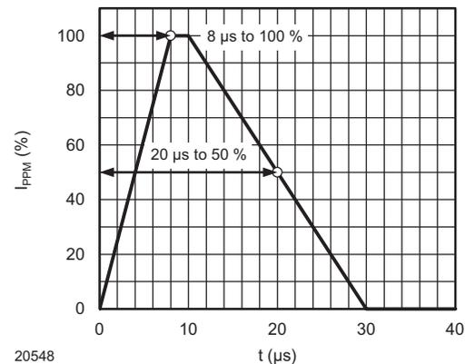
Fig. 2 - 8/20  $\mu\text{s}$  Peak Pulse Current Wave Form
