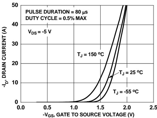
**Figure 5. Transfer Characteristics**
