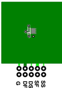
a. 53  $^\circ\text{C}/\text{W}$  when mounted on a 1 in<sup>2</sup> pad of 2 oz copper.
