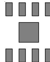
(a) Copper Area = (2.3 x 2.3) mm<sup>2</sup>,  $\theta_{JA} = 75^\circ\text{C/W}$
