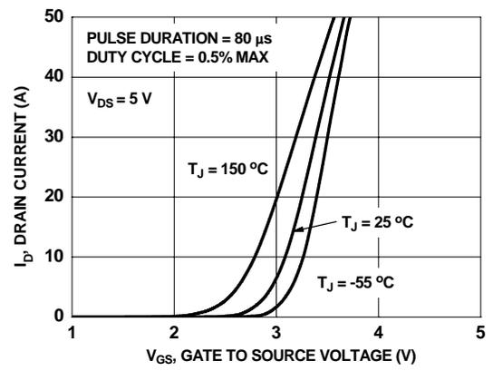
Figure 5. Transfer Characteristics
