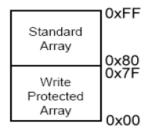
State of the EEPROM memory area after write access to the Protect Register
