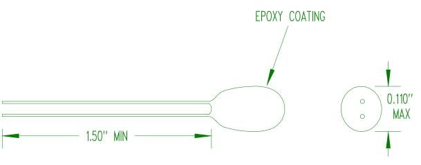
RESISTANCE @  $+25^{\circ}\text{C} = 10,000 \ \Omega \pm 5\%$ RESISTANCE/TEMPERATURE CURVE = ''J''
