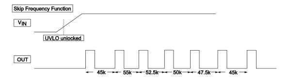
Switching frequency is changed as follows. ...  $\times 0.9 \rightarrow \times 1.1 \rightarrow \times 1.05 \rightarrow \times 1 \rightarrow \times 0.95 \rightarrow \times 0.9 \rightarrow \times 1.1 \dots$  It's repeated by this loop.
