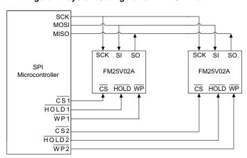
Figure 2. System Configuration with SPI Port
