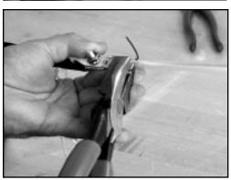
Note: Wind any loose Kevlar™ strands around the lock cap stud for added strain relief before positioning the lock cap onto the extension bracket.
