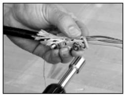
3.11 Making sure that all parts of the connector are kept in alignment, proceed to tighten the lower securing nut completely.
