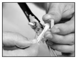
3.10 Position the lock cap from behind onto the extension bracket while capturing either the dielectric or metallic strain members.
