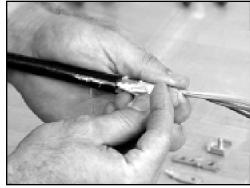
Place the extension bracket over the stud of the connector bottom. Tabs facing up.
