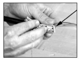
Install second securing nut and tighten down completely.
