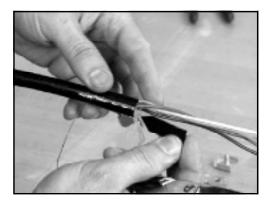
3.5 Install the connector bottom between the cable shield and fiber protector until it stops at the top of the outer sheath opening due to the two outward protruding tabs on the connector bottom. Tap the outer cable sheath in the connector bottom area to set the connector teeth.
