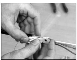
Place the first securing nut on the connector bottom stud and hand tighten.
