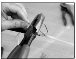
3.9 Crimp wires flat while positioning the ends inside of the tabs on the extension bracket.
