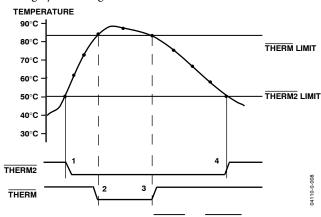
Figure 22. Operation of the THERM and THERM2 Interrupts
