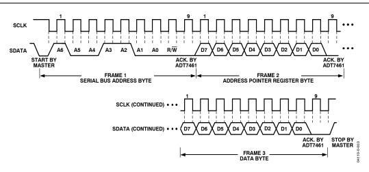
Figure 17. Writing a Register Address to the Address Pointer Register, then Writing Data to the Selected Register
