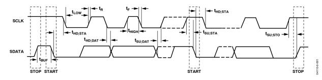
Figure 2. Serial Bus Timing
