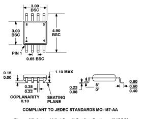
Figure 27. 8-Lead Mini Small Outline Package [MSOP] (RM-8) Dimensions shown in millimeters
