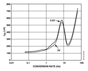
Figure 14. Operating Supply Current vs. Conversion Rate
