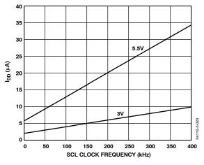
Figure 11. Standby Supply Current vs. Clock Frequency
