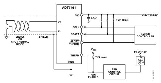
Figure 25. Typical Application Circuit
