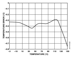
Figure 5. Temperature Error vs. Actual Temperature Using 2N3906
