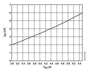
Figure 12. Standby Current vs. Supply Voltage
