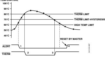
Figure 21. Operation of the ALERT and THERM Interrupts
