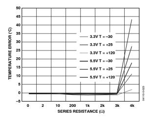
Figure 15. Temperature Error vs. Series Resistance
