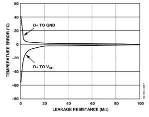
Figure 4. Temperature Error vs. Leakage Resistance
