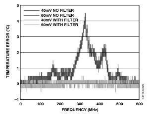
Figure 10. Temperature Error vs. Common-Mode Noise Frequency (With and Without R-C-R Filter of 100  $\Omega$ -2.2 nF-100  $\Omega$ )
