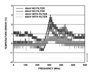
Figure 6. Temperature Error vs. Differential Mode Noise Frequency (With and Without R-C-R Filter of  $100 \Omega - 2.2 \text{ nF} - 100 \Omega$ )
