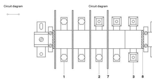
1 = high current connector, AS screw set on both sides 2 = high current connector, terminal sleeve KH on one side, screw set AS on the other side 3 = high current connector, terminal sleeves KH on both sides, for direct cable connection 7 = separating plate 8 = end piece
