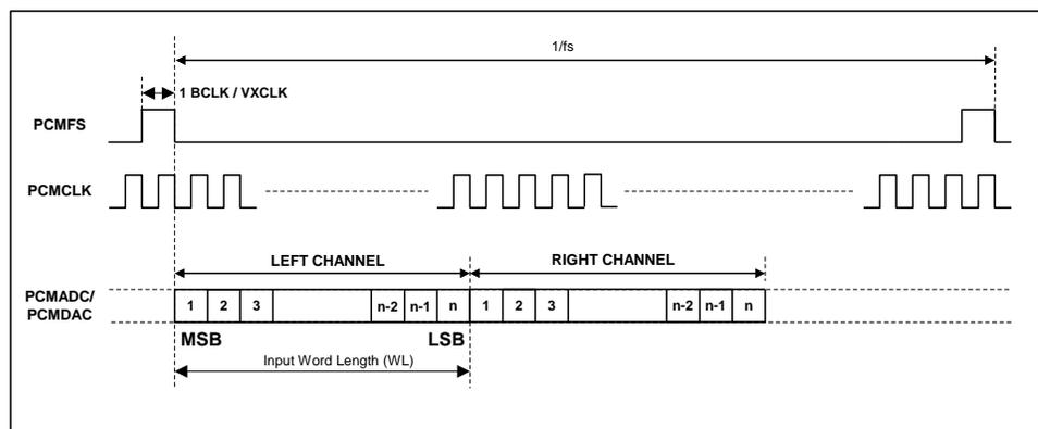
Figure 7 DSP Mode Audio Interface (mode A, FSP=0)
