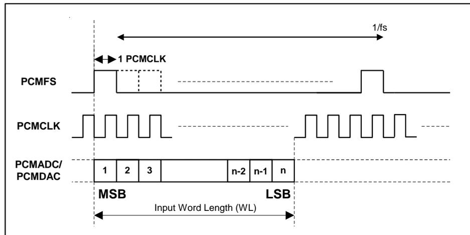
Figure 14 PCM Interface Mono Mode (mode B, FSP=1)
