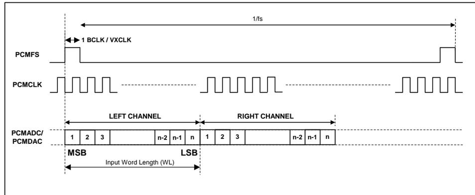
**Figure 15 DSP Mode Audio Interface (mode B, FSP=1)**
