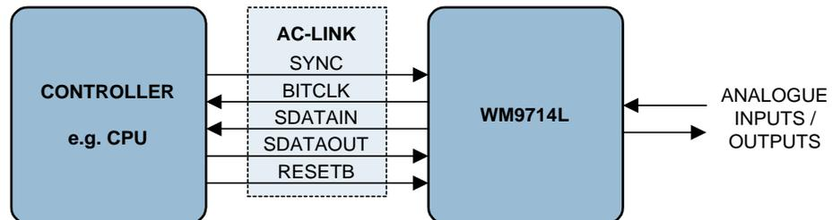
**Figure 12 AC-Link Interface (typical case with BITCLK generated by the AC97 CODEC)**
