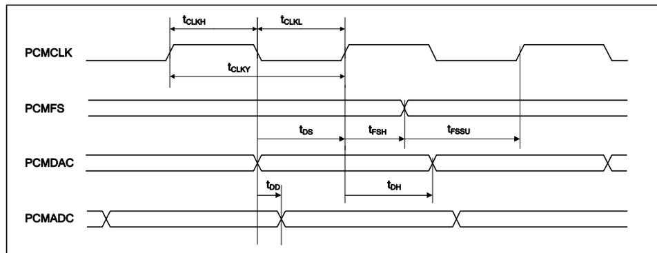
**Figure 7 Digital Audio Data Timing – Slave Mode**
