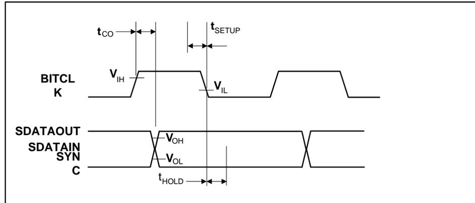
**Figure 2 Data Setup and Hold (50pF External Load)**
