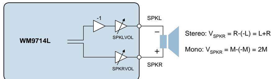
**Figure 32 Speaker Output Connection (INV = 1)**
