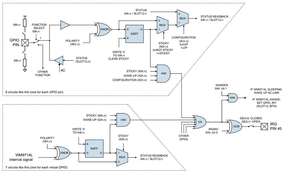
**Figure 27 GPIO Logic**
