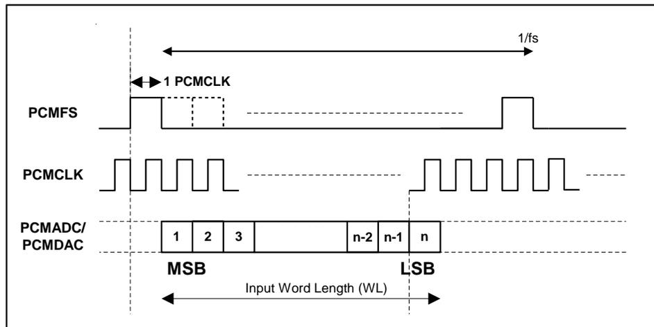
Figure 13 PCM Interface Mono Mode (mode A, FSP=0)
