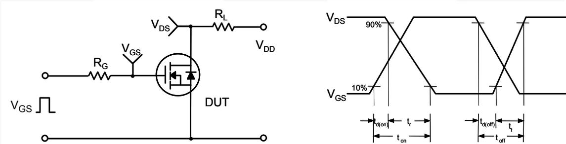
Figure 13. Resistive Switching Test Circuit & Waveforms
