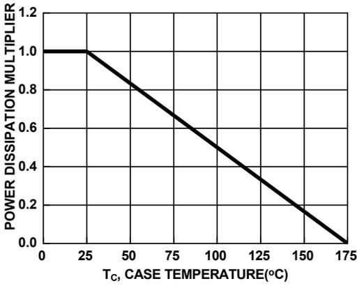
Figure 1. Normalized Power Dissipation vs. Case Temperature
