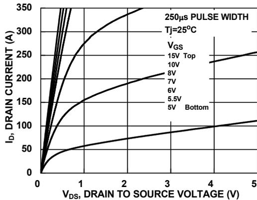
Figure 9. Saturation Characteristics
