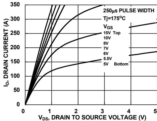
Figure 10. Saturation Characteristics
