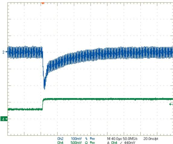
Step Load Transient Response (Vin=12V, Vout=5.0V, Clad=0, Iout=3A to 1.5A)
