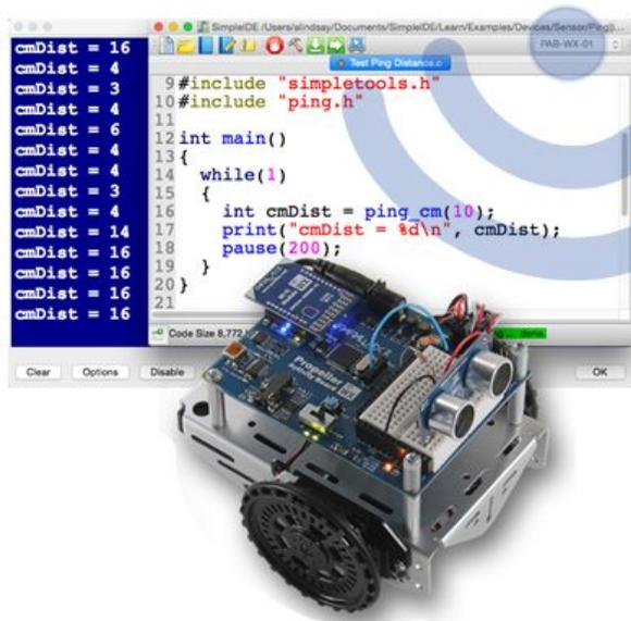
Program the Propeller Activity Board WX over Wi-Fi with the DIP module, and see its remote sensor data display on your computer in real time. This is especially useful when preparing for robot contests because your ActivityBot can roam in a maze and transmit sensor data to the SimpleIDE Terminal without the USB tether. Reprogram it without ever removing it from the maze!
