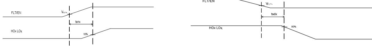
**Figure 10: Output enable/disable timing waveform**
