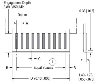
Equal spaces = total number of dual-cavity positions in connector, minus one, times cavity centerline dimension ("A").
