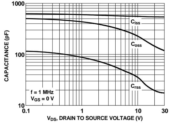
**Figure 8. Capacitance vs Drain to Source Voltage**
