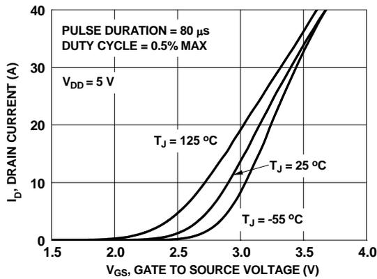
Figure 5. Transfer Characteristics
