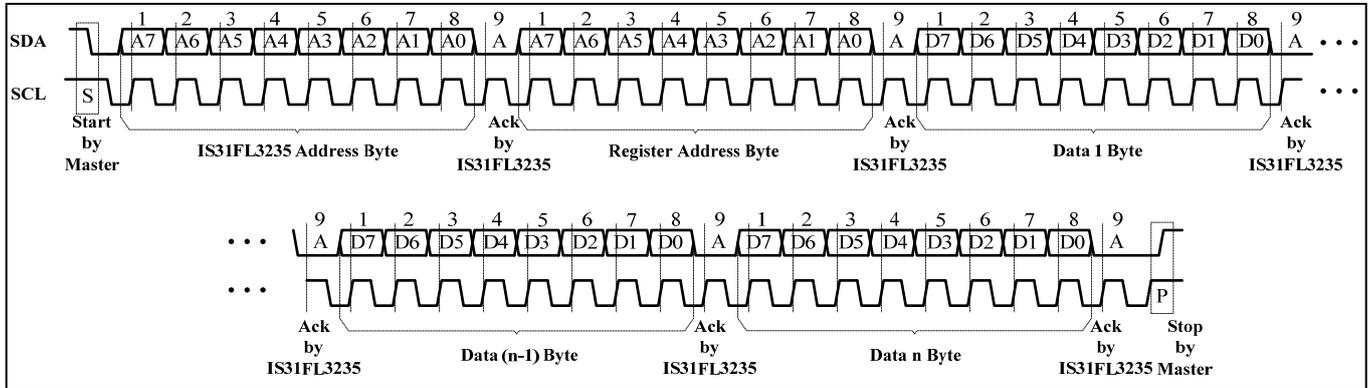
Figure 5 Writing to IS31FL3235(Automatic address increment)
