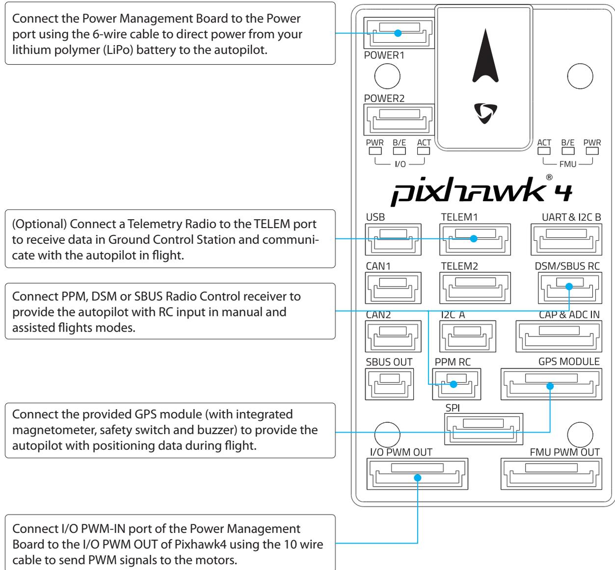
Connect the PMB to the POWER port using the 6-wire cable to direct power from your lithium polymer (LiPo) battery to the autopilot.
