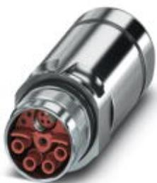
Coupling connector, straight long, shielded: yes, Screw locking, M23, Number of positions: 4+4+4+PE / 3+N +PE, Type of contact: Socket, Crimp connection, Cable diameter: 15 mm ... 18 mm
