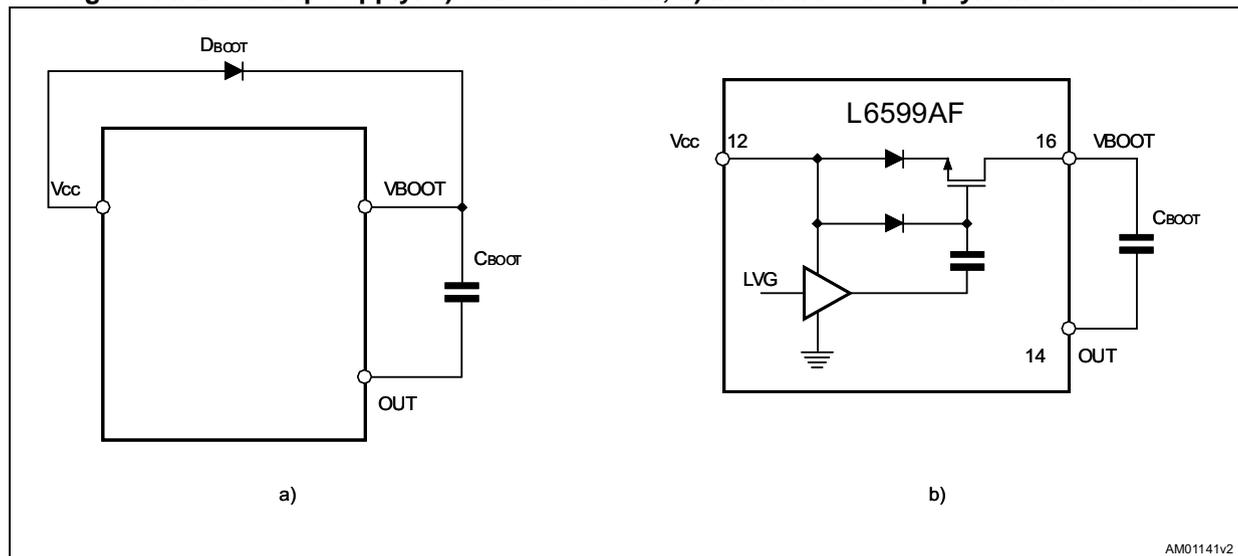
The diode prevents any current being able to flow from the VBOOT pin back to  $V_{CC}$ , in case the supply is quickly turned off when the internal capacitor of the pump is not fully discharged. To drive the synchronous DMOS a voltage higher than the supply voltage  $V_{CC}$  is necessary. This voltage is obtained by means of an internal charge pump ([Figure 14 b](#)).
