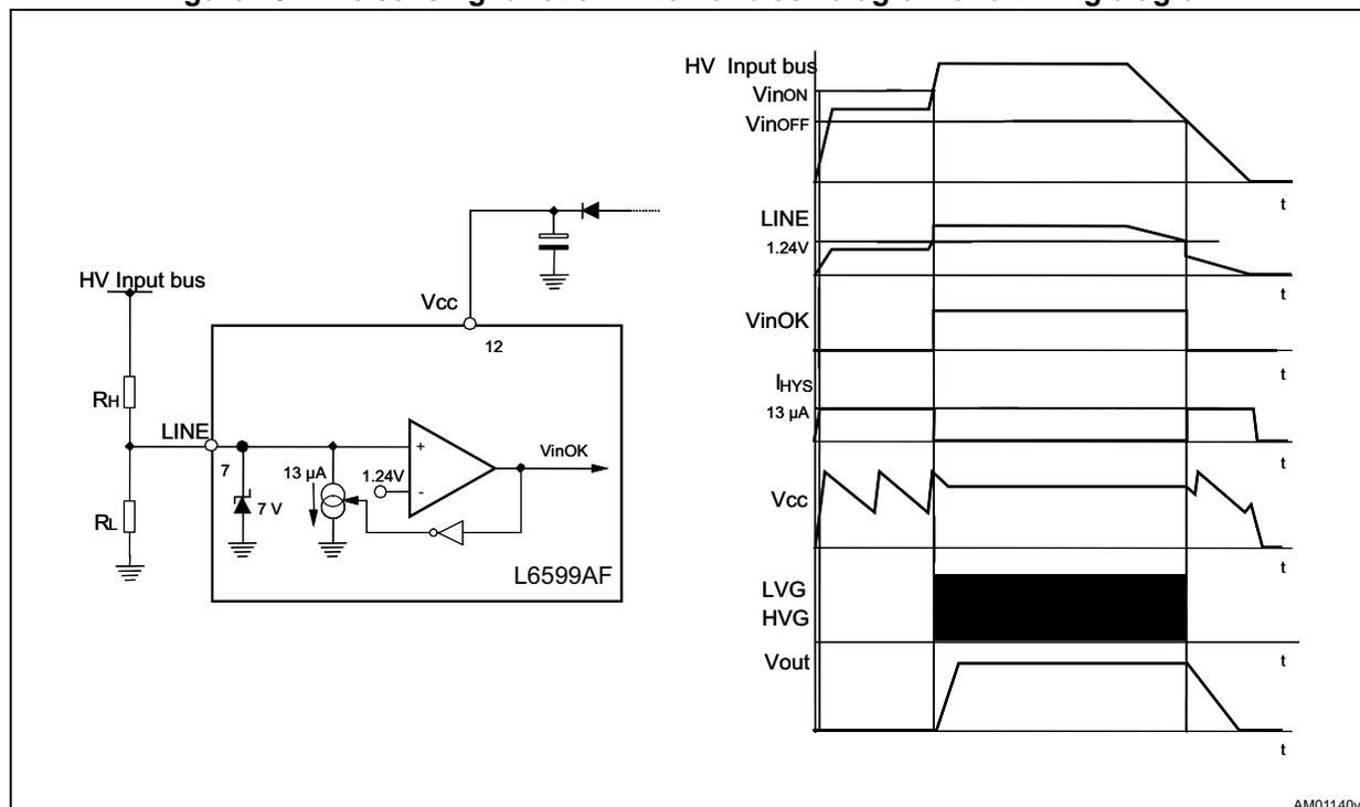
With reference to [Figure 11](#), the following relationships can be established for the ON ( $V_{inON}$ ) and OFF ( $V_{inOFF}$ ) thresholds of the input voltage:
