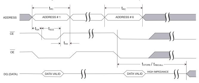
Figure 14. OE Controlled Software STORE/RECALL Cycle [21]
