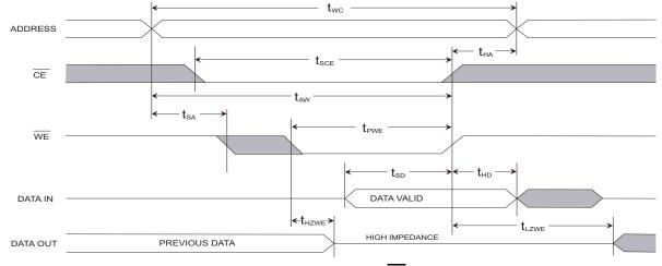
Figure 11. SRAM Write Cycle 2: CE Controlled
