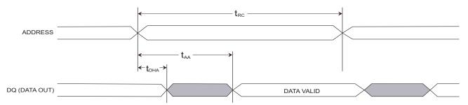
Figure 9. SRAM Read Cycle 2:  $\overline{\text{CE}}$  and  $\overline{\text{OE}}$  Controlled [10, 14]
