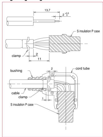
1. The right angle plug can also be assembled by using the same procedure as the straight plug.
