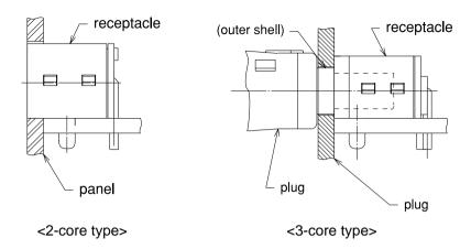
2. After connector assembly, cable must not be pulled over 30N in the arrow-indicated direction. Be careful not to add excessive tensile load because it will lead the damage of connectors.
