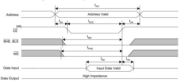
Figure 15. SRAM Write Cycle 2: CE Controlled<sup>[42, 43, 44, 45]</sup>
