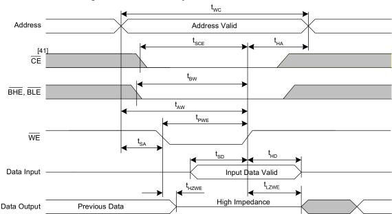
Figure 13. SRAM Write Cycle 1:  $\overline{\text{WE}}$  Controlled [37, 38, 39, 40]
