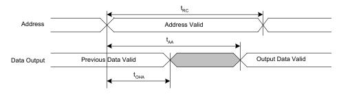
Figure 12. SRAM Read Cycle 2:  $\overline{\text{CE}}$  and  $\overline{\text{OE}}$  Controlled<sup>[32, 34, 35]</sup>
