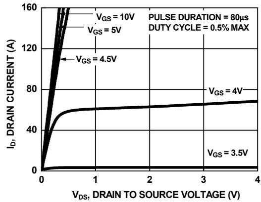
Figure 8. Saturation Characteristics
