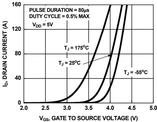
Figure 7. Transfer Characteristics
