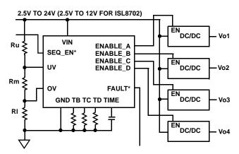
\* SEQ\_EN and FAULT are not available on ISL8700 and ISL8701 FIGURE 1. ISL870x IMPLEMENTATION
