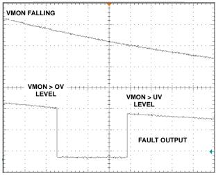
FIGURE 7. VMONITOR FALLING TO FAULT
