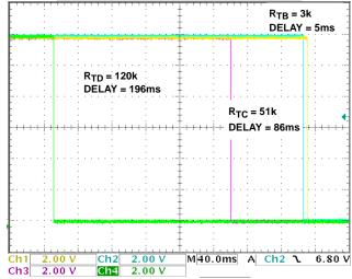
FIGURE 8. ENABLE\_X TO ENABLE\_X ENABLING
