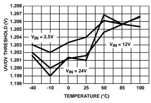
FIGURE 4. UV/OV RISING THRESHOLD
