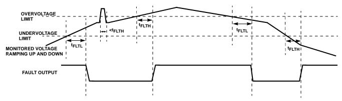
FIGURE 3. ISL8702 FAULT OPERATIONAL DIAGRAM
