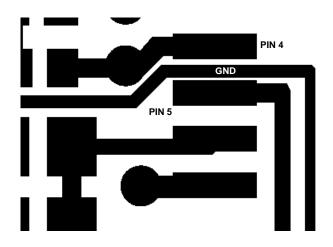
FIGURE 14. LAYOUT DETAIL OF GND BETWEEN PINS 4 AND 5
