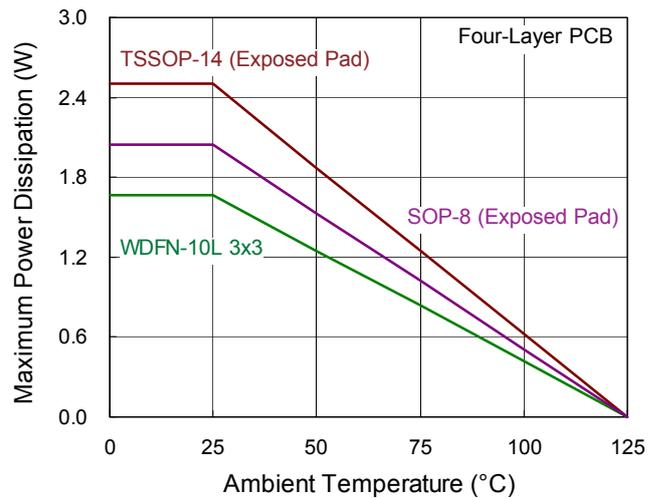
Figure 6. Derating Curve of Maximum Power Dissipation
