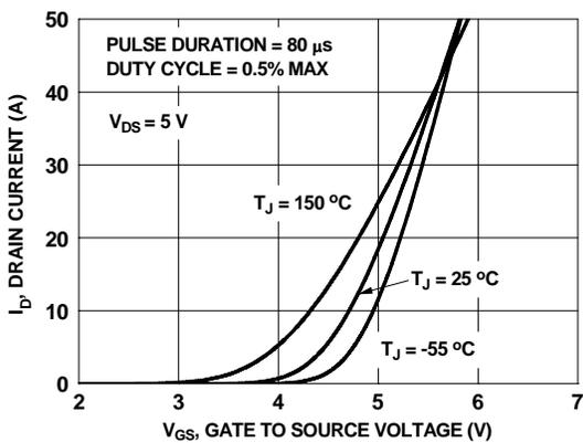
**Figure 5. Transfer Characteristics**
