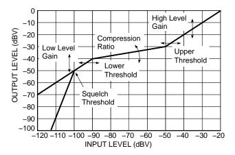
Figure 4. Independent Channel I/O Curve Flexibility
