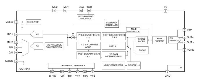
Figure 1. Hybrid Block Diagram
