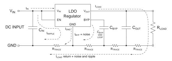
Figure 1: Common LDO Regulator Layout with  $C_{\mbox{\scriptsize BYP}}$  Ripple Feedback Loop.
