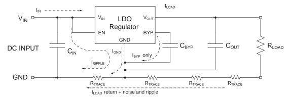
Figure 2: Recommended LDO Regulator Layout.
