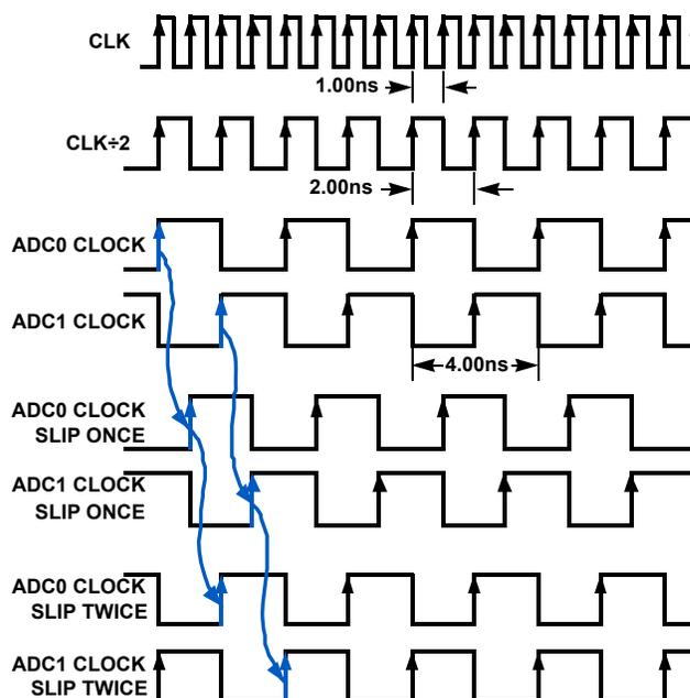
**FIGURE 39. PHASE SLIP: CLK+2 MODE,  $f_{\text{CLK}} = 1000\text{MHz}$**
