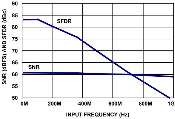
FIGURE 4. SNR AND SFDR vs f<sub>IN</sub>
