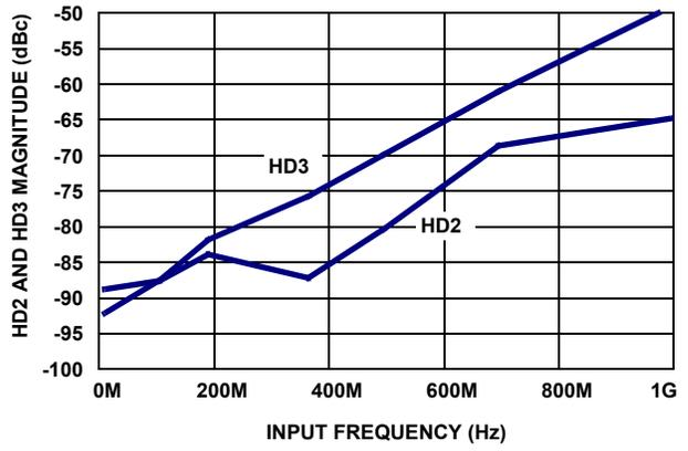
FIGURE 5. HD2 AND HD3 vs f<sub>IN</sub>
