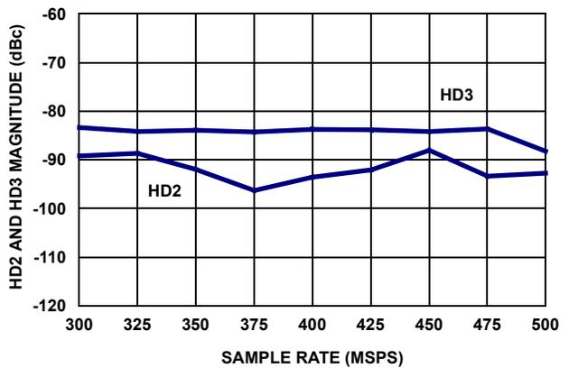
FIGURE 9. HD2 AND HD3 vs f<sub>SAMPLE</sub>
