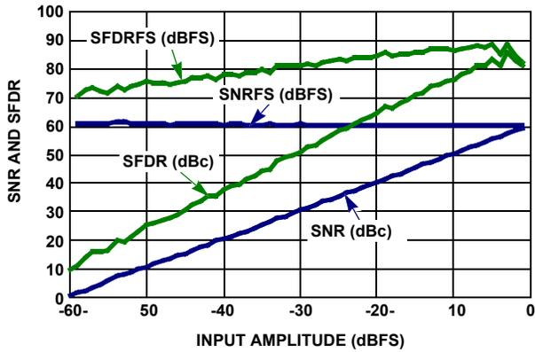
FIGURE 6. SNR AND SFDR vs A<sub>IN</sub>
