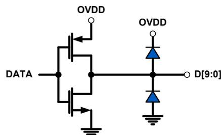
FIGURE 46. CMOS OUTPUTS
