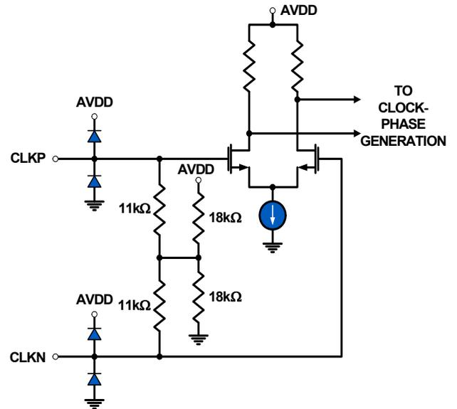
FIGURE 42. CLOCK INPUTS
