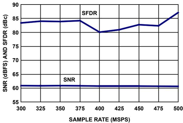
FIGURE 8. SNR AND SFDR vs f<sub>SAMPLE</sub>
