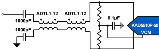
FIGURE 27. TRANSMISSION-LINE TRANSFORMER INPUT FOR HIGH IF APPLICATIONS
