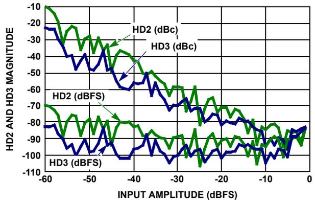
FIGURE 7. HD2 AND HD3 vs A<sub>IN</sub>
