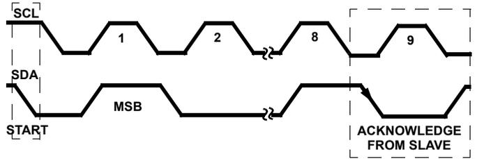
FIGURE 4. ACKNOWLEDGE ON THE I<sup>2</sup>C BUS
