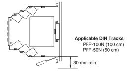
Leave at least 30 mm of space between the product and other devices to allow easy installation and removal.
