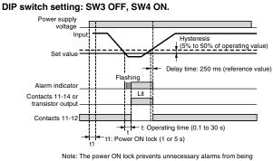
Note: The power ON lock prevents unnecessary alarms from being generated during the instable period when the power is first turned on. There is no relay output during timer operation.
