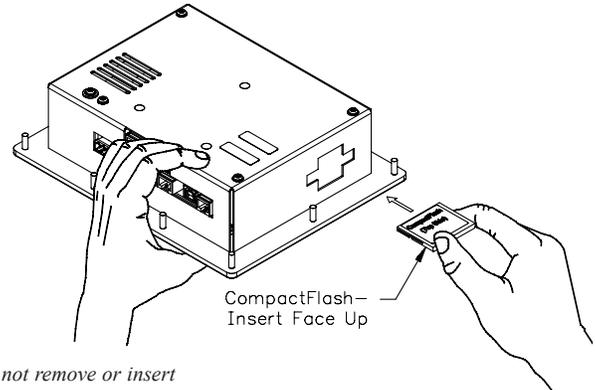
*Note: Do not remove or insert the CompactFlash card while power is applied. Refer to "Front Panel LEDs."*
