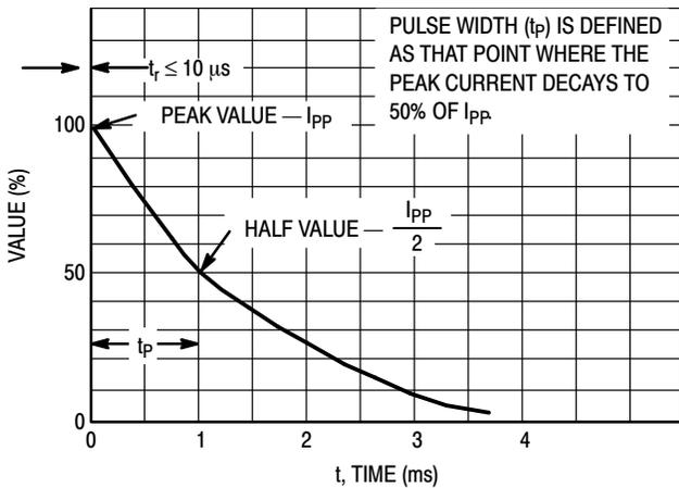
Figure 4. Pulse Waveform
