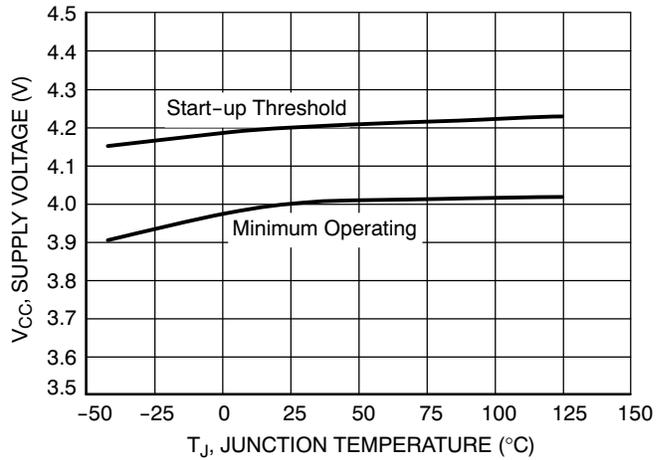
**Figure 4. Supply Voltage Thresholds vs. Junction Temperature**
