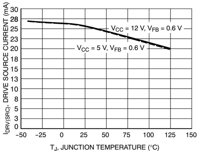
**Figure 7. Drive Source Current vs. Junction Temperature**
