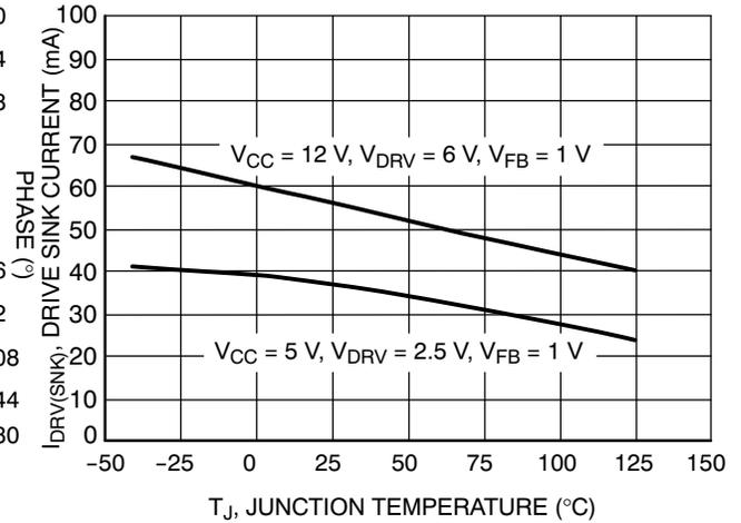
**Figure 6. Drive Sink Current vs. Junction Temperature**
