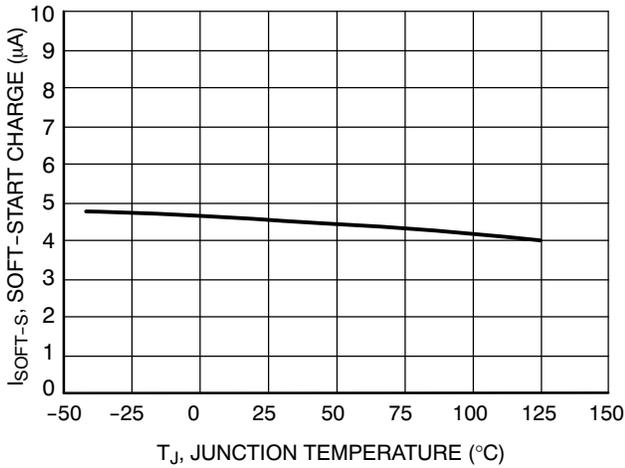
**Figure 9. Soft-Start Charge Current vs. Junction Temperature**
