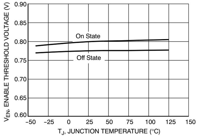
**Figure 10. Enable Threshold Voltages vs. Junction Temperature**
