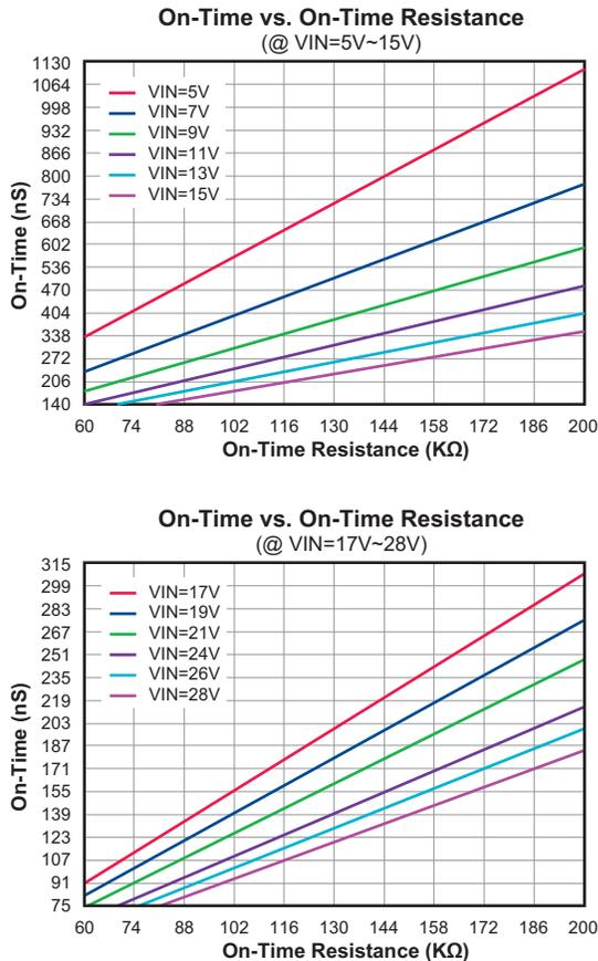
Figure 3. T<sub>ON</sub> vs. R<sub>TON</sub> Curves for AOZ2261QI-15
