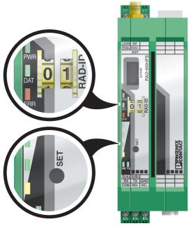
Figure 3 Display and diagnostic elements
