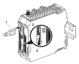
Figure 14 Configuration via CONFSTICK
