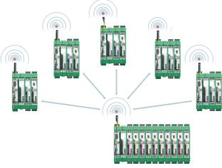
Figure 16 Example of multipoint-to-point connection
