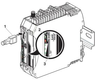
Figure 12 Antenna connection
