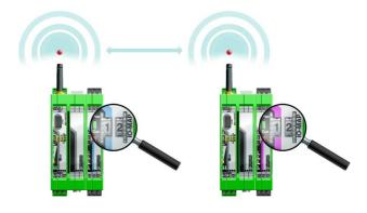
Figure 13 Example: 2 RAD-DAIO6-IFS with the same address
