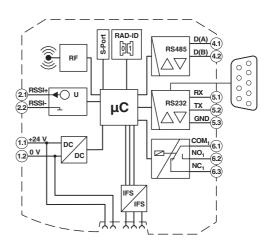
Figure 2 Circuit diagram
