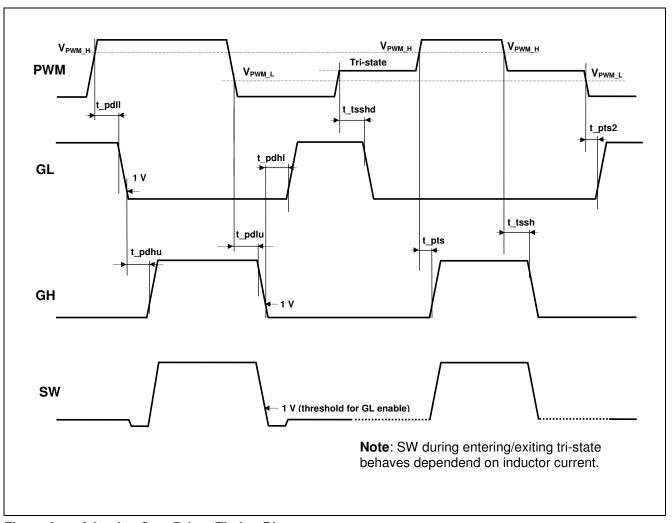
Figure 8 Adaptive Gate Driver Timing Diagram
