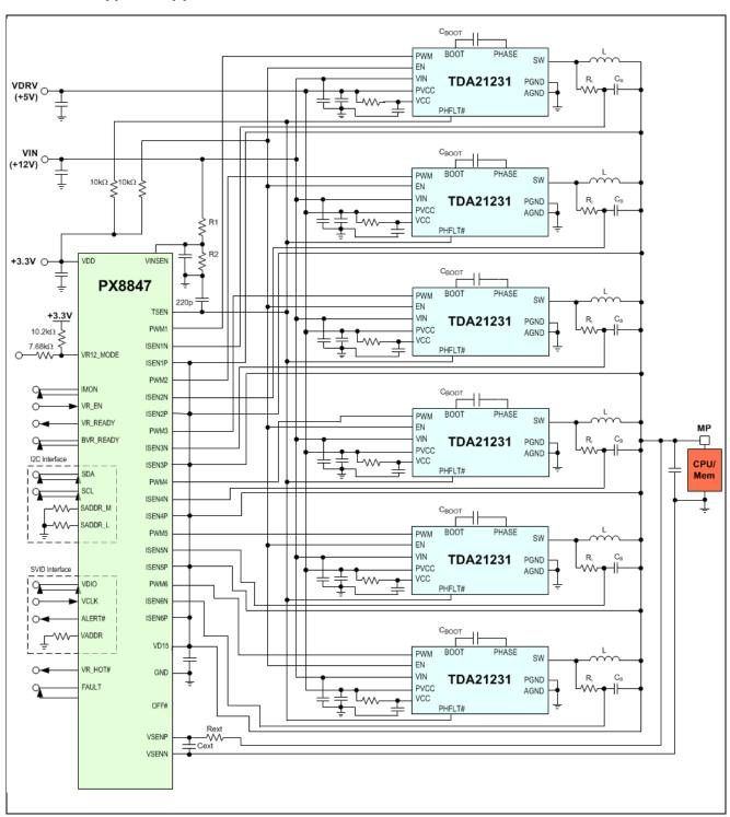
Figure 7 Six-phase voltage regulator - typical application (simplified schematic)
