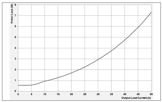
Figure 12 Power Loss at VIN = 12 V, VCC = PVCC = 5 V,  $f_{SW}$  = 600 kHz, VOUT = 1.8 V
