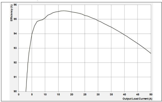
Figure 11 Efficiency at VIN = 12 V, VCC = PVCC = 5 V, f<sub>SW</sub> = 600 kHz, VOUT = 1.8 V
