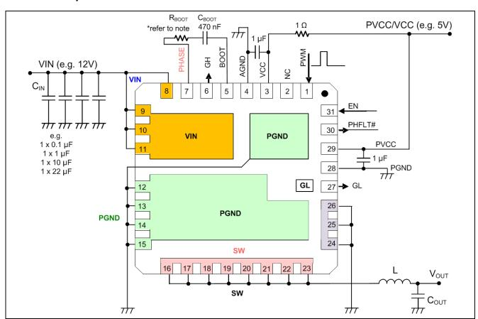
Figure 6 Pin Interconnection Outline (example, transparent top view)
