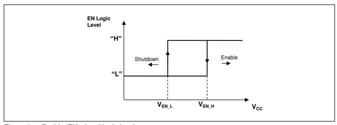
Figure 4 Enable (EN) signal logic levels
