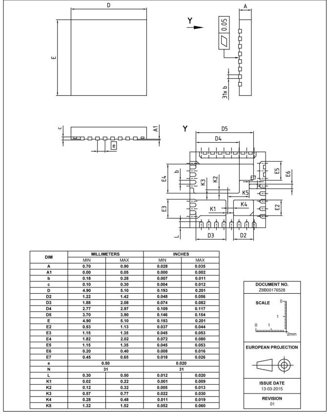
Figure 13 Mechanical Dimensions (in mm)
