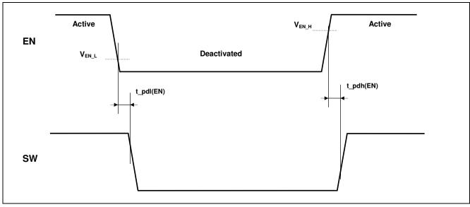
Figure 9 EN Timing Diagram
