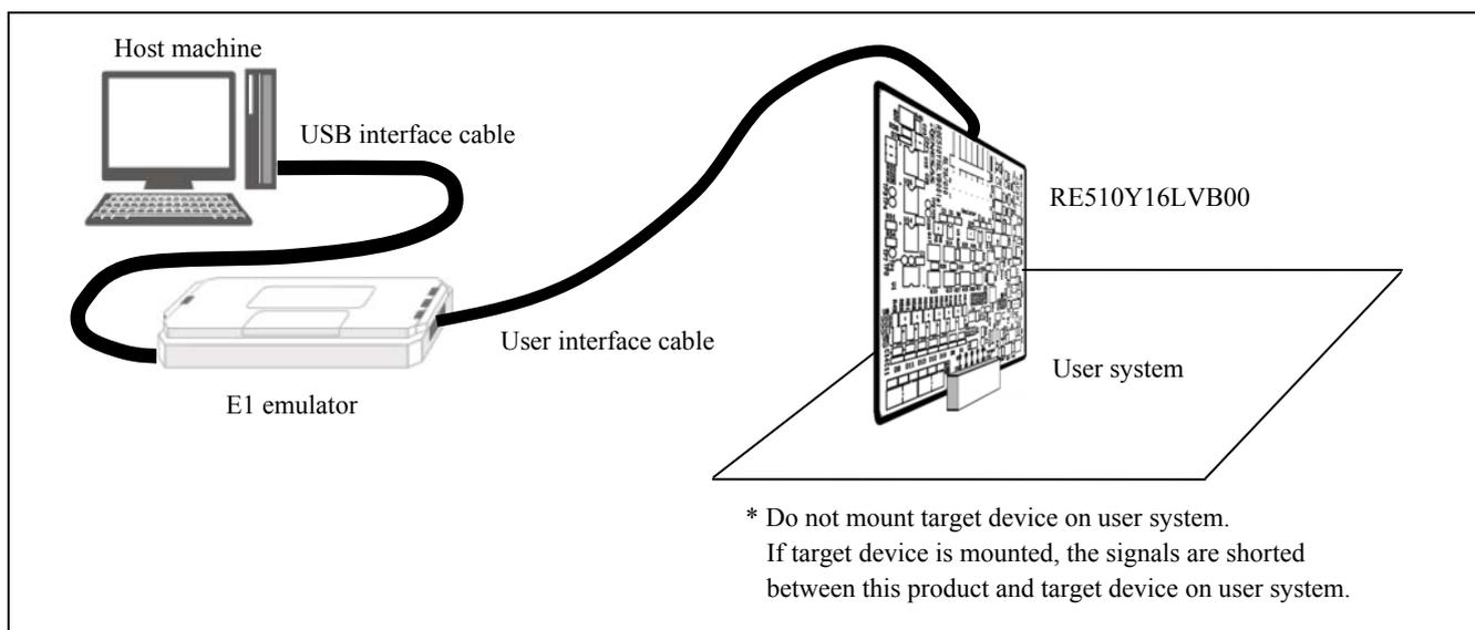
Figure 1 System Configuration
