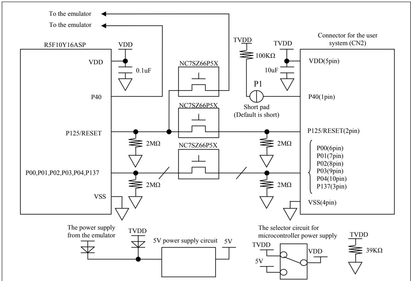
Figure 3 Internal circuit of this product (R0E510YLVB00)
