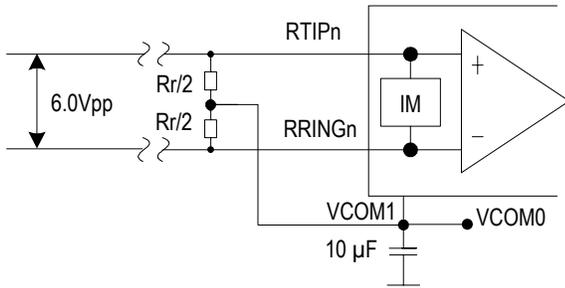
**Note:** 1. Two Rr/2 resistors should be connected to VCOM[1:0] that are coupled to ground via a 10 µF capacitor, which provide 60 Ω common mode input resistance.
