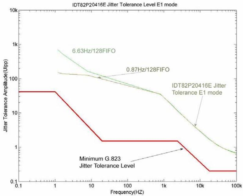
Figure-41 E1 Jitter Tolerance Performance
