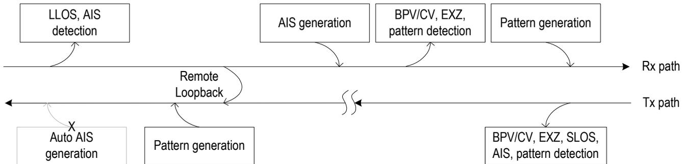
**Figure-26 Priority Of Diagnostic Facilities During Manual Remote Loopback**
