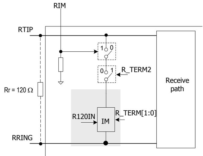
**Figure-3 Switch between Impedance Matching Modes**
