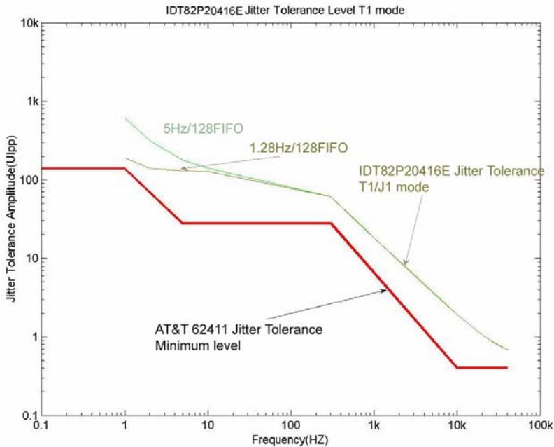
Figure-42 T1/J1 Jitter Tolerance Performance
