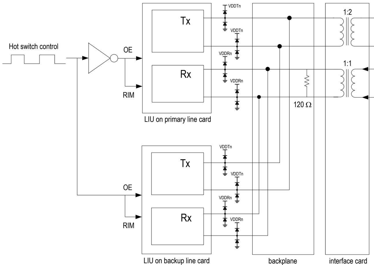
**Rx:** Partially Internal Impedance Matching mode. A fixed external 120 Ω resistor is placed on the backplane and provides a common termination for T1/J1/E1 applications. The R\_TERM[2:0] bits (b2~0, RCF0,...) setting is as follows: '000' for T1 100 Ω twisted pair cable, '001' for J1 110 Ω twisted pair cable, '010' for E1 120 Ω twisted pair cable and '011' for E1 75 Ω coaxial cable.
