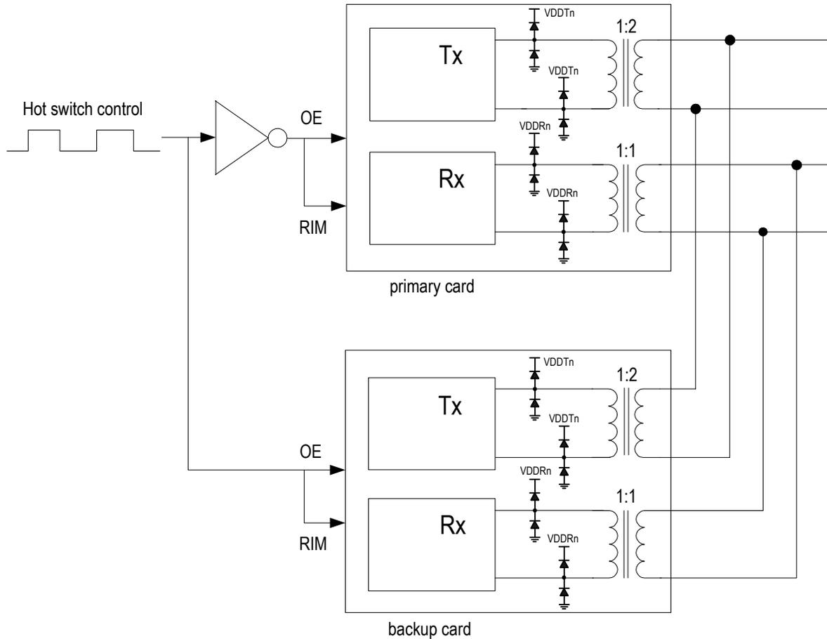
**Rx:** Fully Internal Impedance Matching mode. In this mode, there is no external resistor required. The R\_TERM[2:0] bits (b2~0, RCF0,...) setting is as follows: '000' for T1 100Ω twisted pair cable, '001' for J1 110 Ω twisted pair cable, '010' for E1 120 Ω twisted pair cable and '011' for E1 75 Ω coaxial cable.
