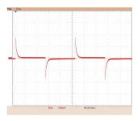
Figure 14. Load Regulation (I<sub>out</sub> changing from 10% to 100%–0.3 A to 3.0 A)
