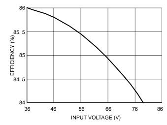
Figure 7. DC/DC Converter Efficiency vs. Input Voltage
