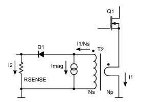
Figure 2. Implementation of the Current Sense Transformer
