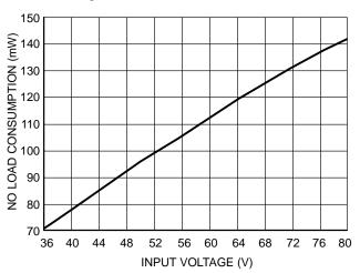
Figure 9. No Load Consumption vs. Input Voltage
