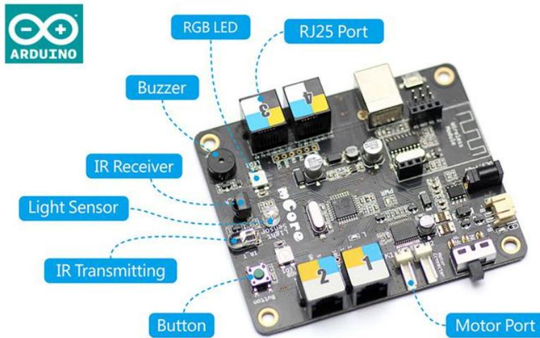
Arduino is an open-source electronic prototyping platform used by people in the global world to start a project quickly. It has been proved to be very expandable and suitable for beginners. So we designed mBot's electronics based on Arduino platform, which is easy for kids to use and extend, and bring their every idea to life.
