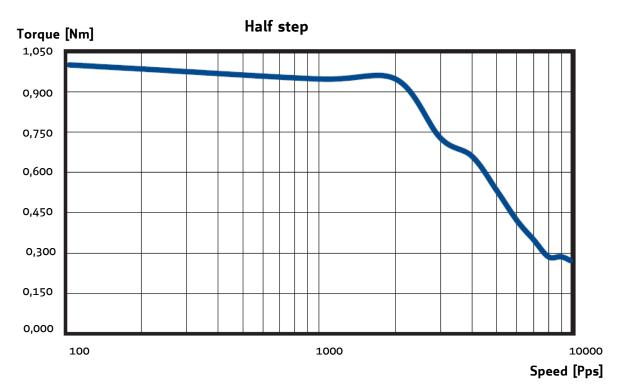
Figure 5.2: QSH-5718-51-28-101 speed vs. torque characteristics
