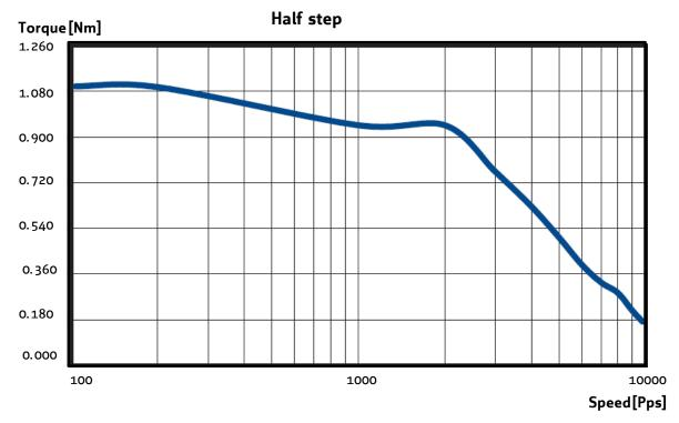
Figure 5.3: QSH5718-56-28-126 speed vs. torque characteristics
