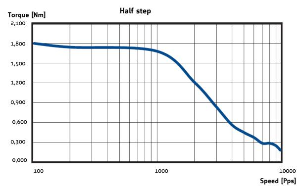
Figure 5.4: QSH5718-76-28-189 speed vs. torque characteristics
