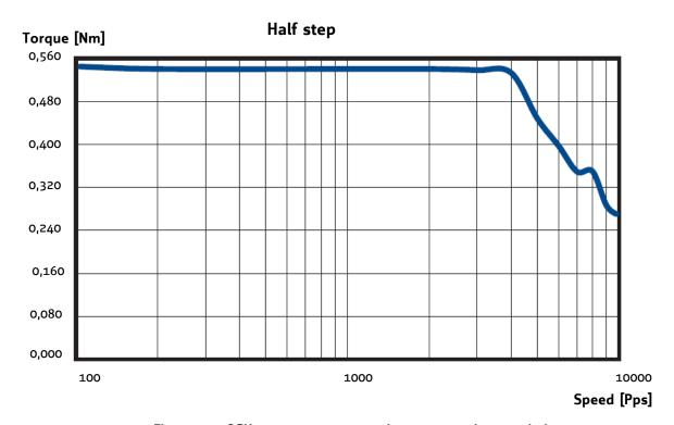
Figure 5.1: QSH5718-41-28-055 speed vs. torque characteristics
