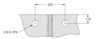
RECOMMENDED PCB LAYOUT NOTE: THIS PATTERN IS FOR REFERENCE ONLY. PATTERN MAY VARY DEPENDING ON BOARD TYPE, SPECIFIC ELECTRICAL OR MECHANICAL REQUIREMENTS.
