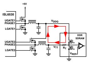
FIGURE 6. V<sub>TT</sub> CURRENT SINKING LOOP
