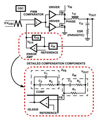
FIGURE 8. VOLTAGE-MODE BUCK CONVERTER COMPENSATION DESIGN
