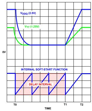
FIGURE 5. OVERCURRENT PROTECTION RESPONSE
