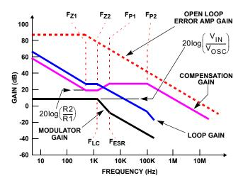
FIGURE 9. ASYMPTOTIC BODE PLOT OF CONVERTER GAIN
