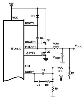
FIGURE 3. OUTPUT VOLTAGE SELECTION OF VDDQ
